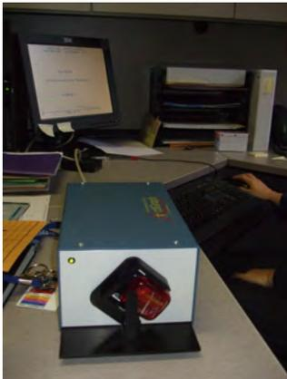
Before each test, all devices are verified (calibrated) to ensure that measures are perfect! Here you can see the accelerometer being verified.
